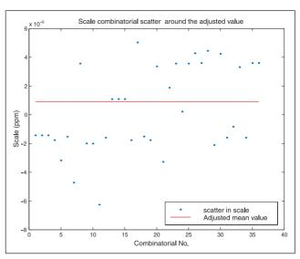
Fig. 3: Scatter of the 36 combinatorial solutions of scale around adjusted value
