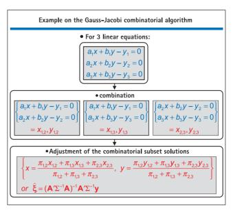
Fig. 2: Example of application of Gauss-Jacobi algorithm
