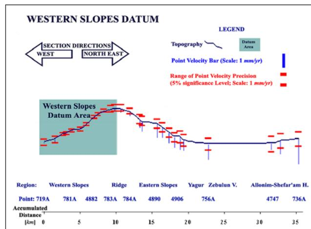
Fig. 3: Extended solution of the leveling network weighted by the Carmel western slopes datum. A significant BM velocity (mm per year) appears where the velocity line deviates from the precision margins at a 5% significance level.
