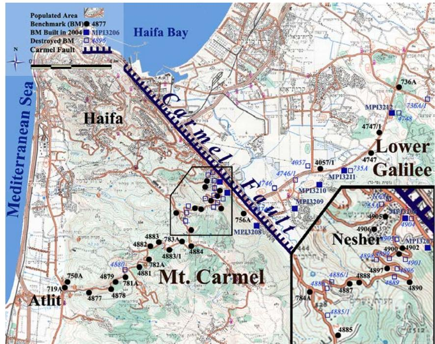
Precise leveling measured by the SOI in 1987 in the extended part was used, in order to utilize the measuring data from 2003 for movement analysis. That data was taken from the original books kept in the SOI archive.
