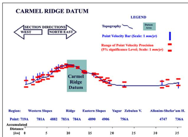
Fig. 4: Extended solution of the leveling network weighted by the Carmel ridge datum. A significant BM velocity appears where the velocity line deviates from the precision margins at a 5 % significance level.
