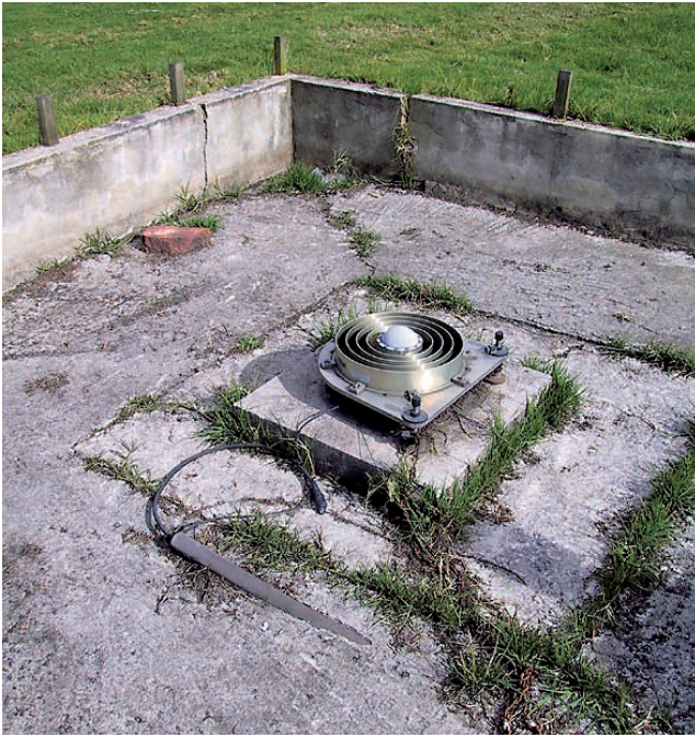
Fig. 5: Antenna set-up at the BOGT station
