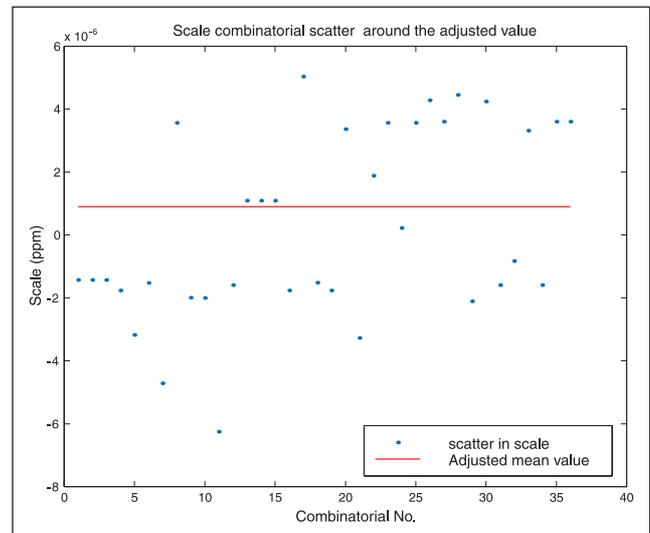
Fig. 3: Scatter of the 36 combinatorial solutions of scale around adjusted value
