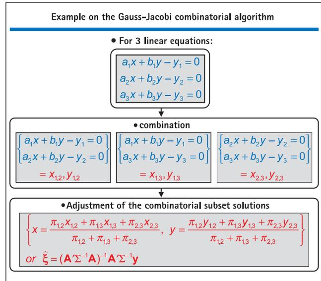
Fig. 2: Example of application of Gauss-Jacobi algorithm
