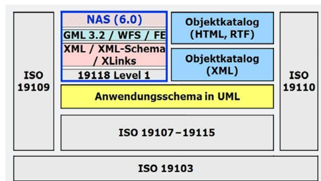
Fig. 8: AAA®-embedding existing international standards (AdV 2008) (NAS = exchange interface, Objektkatalog = feature catalogue, Anwendungsschema = application schema)
