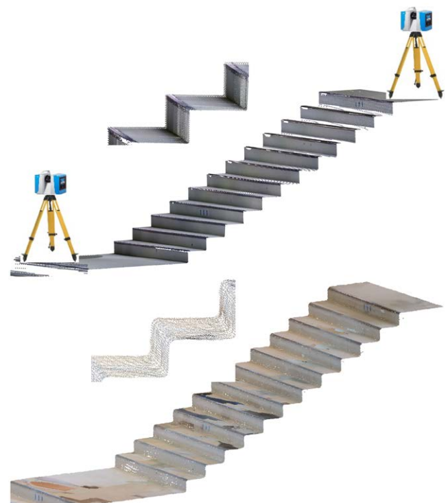
Fig. 7: A small section of the stairs connecting first floor to the ground floor, captured by the TLS (top) and NavVis VLX (bottom)
